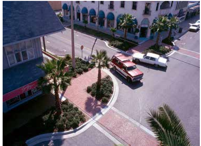
Image 1 - Rounded corner at intersection allows smooth flow of pedestrian activity.
