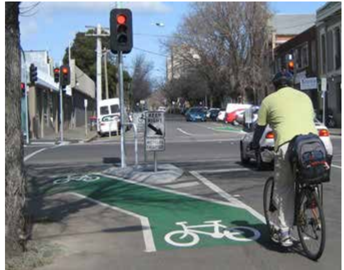
Image 2 - Colored bike lane to indicate safe left-turning point at intersection.
