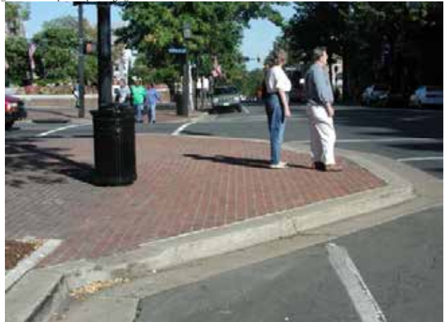
Image 5 - A bulb-out intersection allowing the pedestrian to be clearly seen by oncoming traffic.
