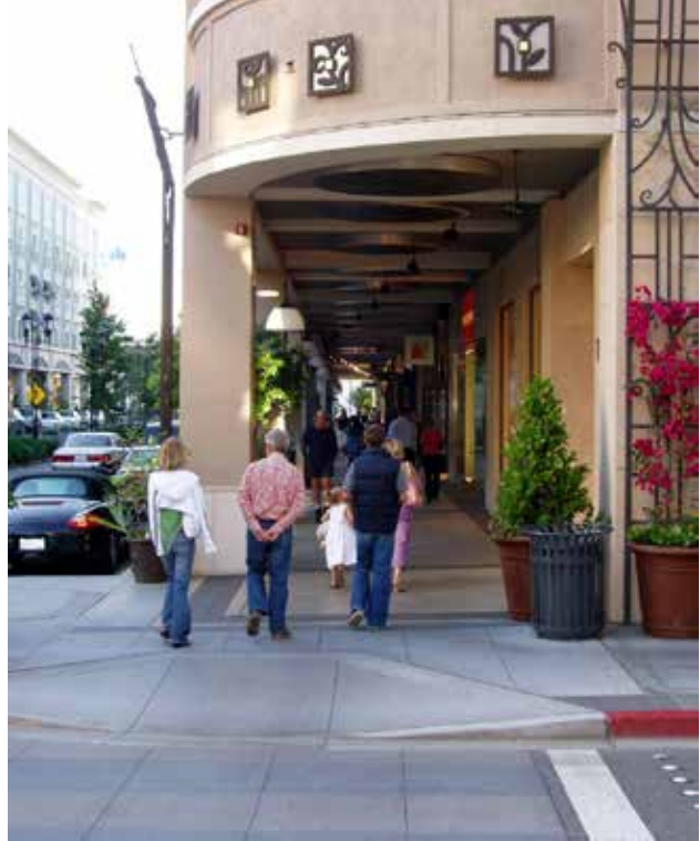
Image 4 - Bulb-out intersection with a continued paving for the crosswalk that is separate from the asphalt paving of the street.
