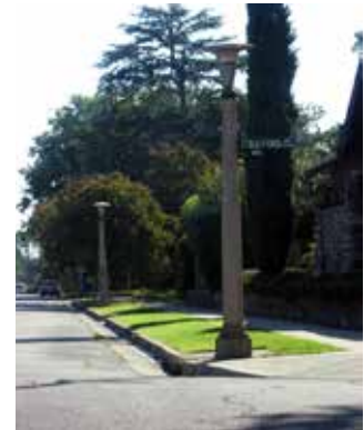
Image 5 - Residential Street with fully shielded lamp post in parkway utilizing post for signage
