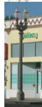
Image 8 - Multi-fixture lamp is appropriate for higher density retail areas (T5 to T6)
